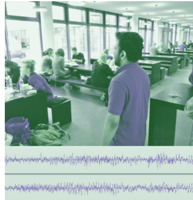
Fig. 2 Sound pressure on the eardrums (above: left ear, below: right ear), recorded with probe microphones in the ears of the person in the foreground, sequence of 1/3 second. Within the depicted snippet at least three distinct auditory objects (voices) in different directions and distances before a complex and noisy background are audible.
