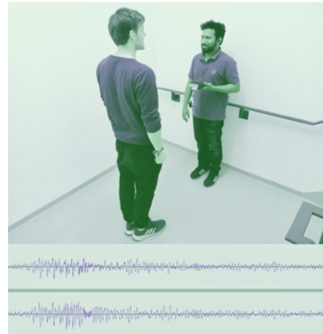
Fig. 1 Sound pressure on the eardrums (above: left ear, below: right ear), recorded with probe microphones in the ears of the person to the right, sequence of 1/3 second. In the depicted snippet – the word <quick> spoken by the person to the left – the voice is clearly audible as a distinct auditory object, close in front within a quiet and very remarkable reflective/resonant acoustical environment.
